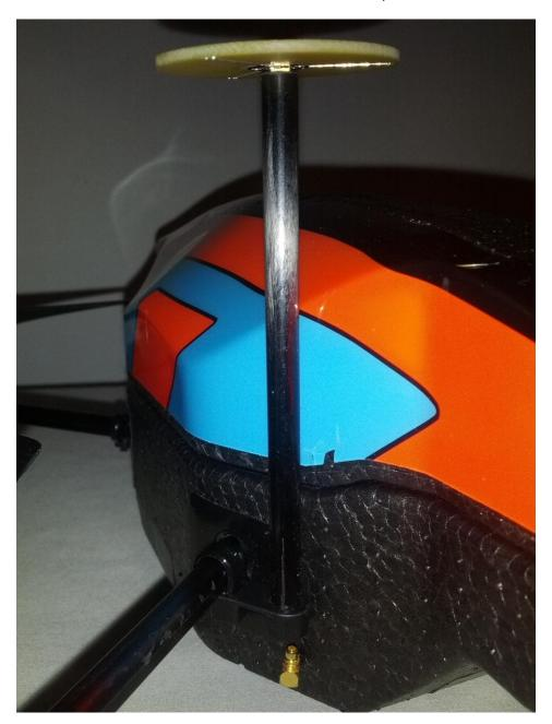
**Bottom Mount – In Flight:** (Velcro used to secure to Bottom Cover)
